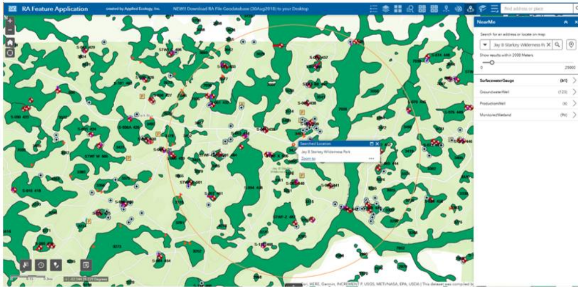
Figure 7.6: Example Using the NearMe Tool in the RAGIS Application, Calculating the Number of Gages and Wells Around a Wetland Site on J.B. Starkey Wellfield.
