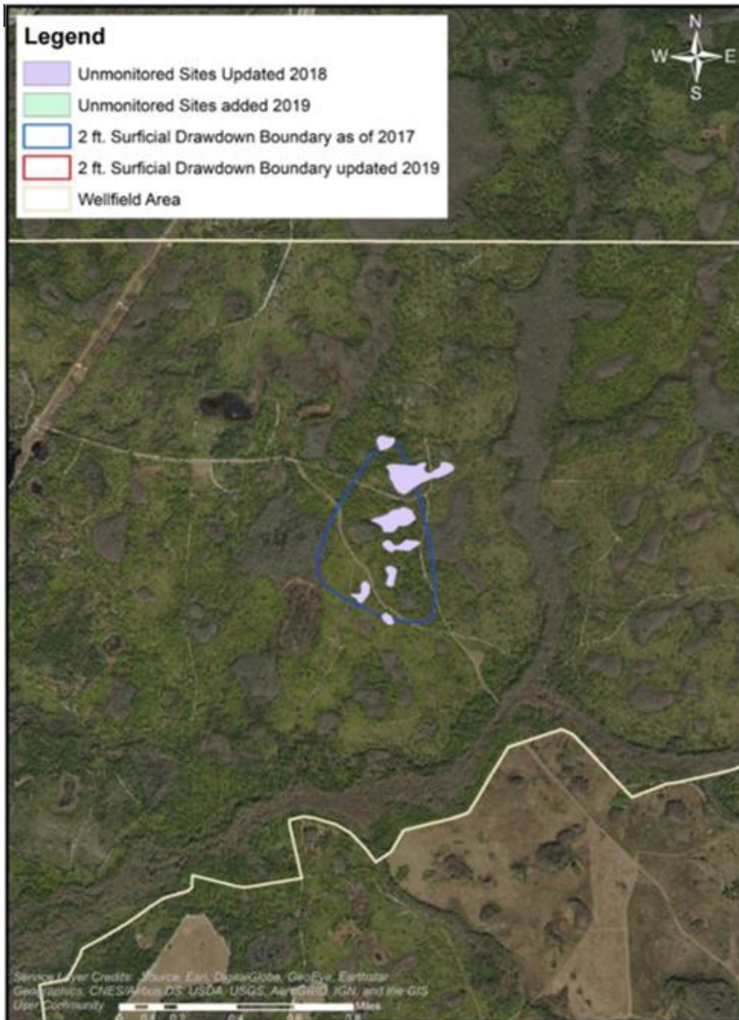
Figure 10.8: Map comparing the 749 wetland sites updated in the 2017 analysis to the 845 finalized from the 2019 pumping analysis, along with the 2017 updated AOI compared with the area developed from 2017 and 2018 pumping for the J.B. Starkey Wellfield. The new AOI is represented by the outermost extent of both the red and blue contours.
